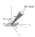
Spectral intensity of radiation  $I_{\lambda}$  is the rate of radiation energy transferred through the differential area dA in the differential solid angle  $d\omega$ around the direction  $\vec{\Omega} = (\theta, \phi)$ in the wavelength  $d\lambda$  about  $\lambda$
