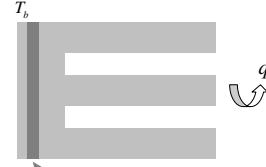
$$q = \frac{T_b - T_\infty}{R_{t,c} + R_{base} + R_{t,o}}$$
