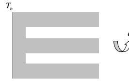
$$q = \frac{T_b - T_\infty}{R_{base} + R_{t,o}}$$
